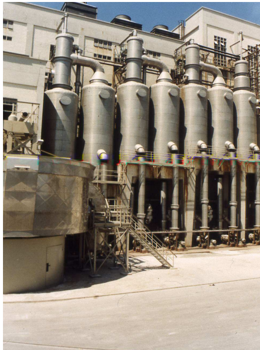
Fig. 4. Barometric installation of flash evaporators at the Bad Friedrichshall salt factory (1969-1995)
